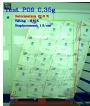
Dynamic deformation P9 to 0.35 g
