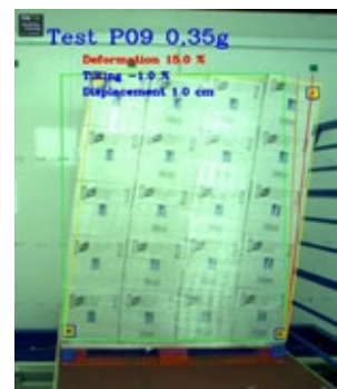
Final deformation P9 at 0.35 g
